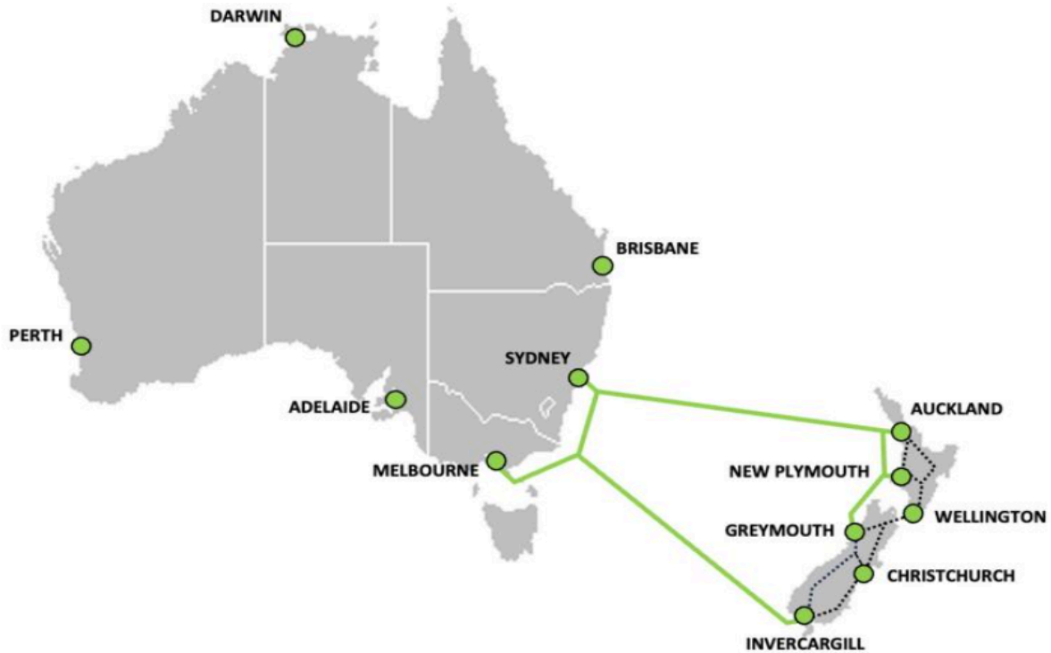
Figure 3. The Tasman Ring Subsea Cable Topology
